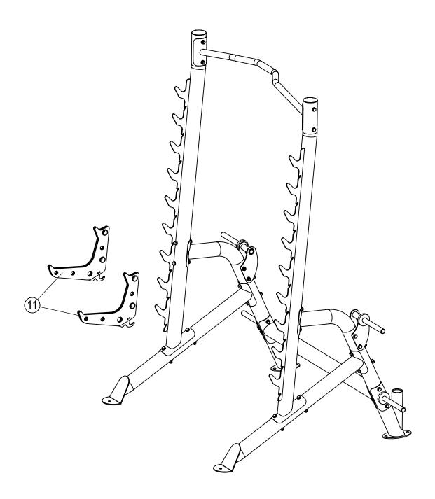
A Add the Spotter Assembly (11) onto the squat rack at the position most comfortable for use.
